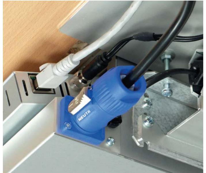
Here you can see the needed connections between the connector panels.
